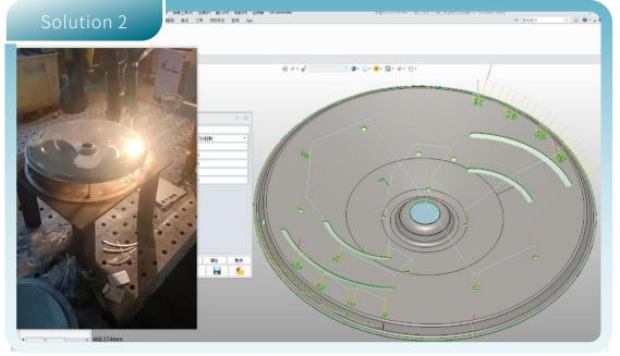
Uses processing solutions to quickly generate high-precision cutting trajectories, verify through physical processing simulation, import CL programs to convert into robot processing points, and optimize paths.
