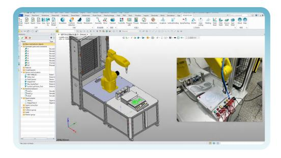
Visually simulates robot trajectory operation, real-time detection of path accessibility, singularity, and collision risks.
