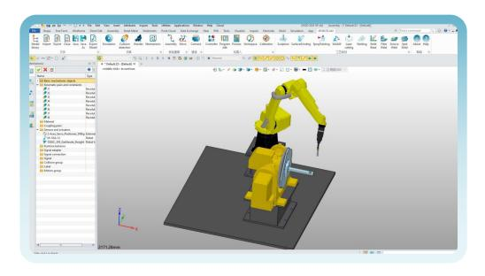
Uses CAD features for workpiece positioning, automatically generates multi-axis machining trajectories, and supports complex engraving applications for robots with 7+ axes.
